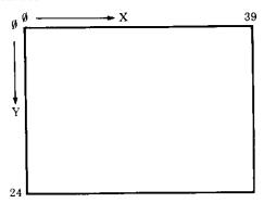
The cursor may be positioned to any part of the screen with the TAB(X,Y) command, thus the following program prints out a diagonal line of As.
