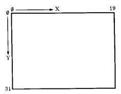
29 This code is used to move the graphics origin. The statement **VDU29** is followed by two numbers giving the X and Y coordinates of the new origin. The graphics screen is addressed
