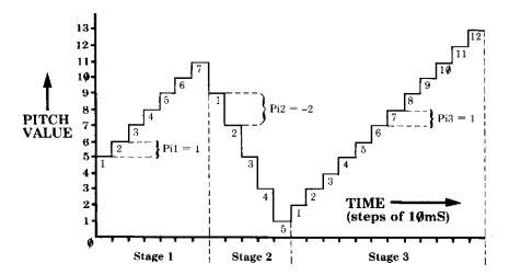
The total time taken for this **ENVELOPE** command is  $10mS \times total$  number of pitch changes, or  $24 \times 0.01$  seconds, = 0.24 seconds. So the **ENVELOPE** is repeated over and over again, until the **SOUND** command finishes.
