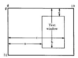
Nothing outside the text window is affected by text commands, such as screen clearing, scrolling, cursor positioning etc. Note that the **TAB(X,Y)** measures from the position of the top left of the current window. Try the following program
