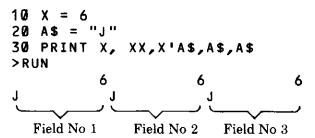
Each field of ten characters width is shown above. As you can see, numbers are printed out to the right of each field, characters to the left. This is done so that numbers line up in the units column, or the least significant decimal.
