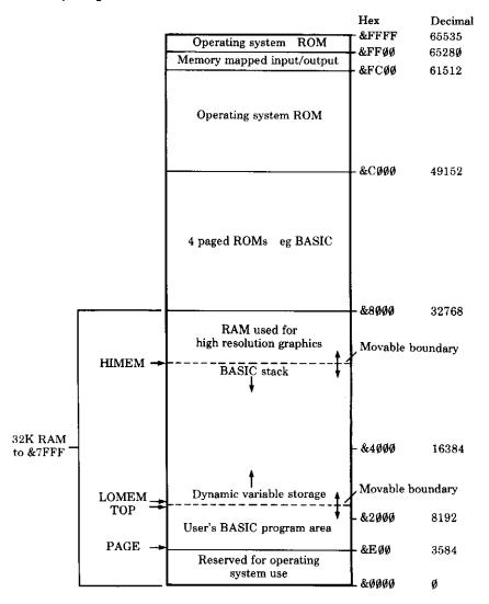
The last address pointer is **HIMEM**. **HIMEM** shows the position of the bottom of the screen memory, so any program or variables must be kept below this value.
