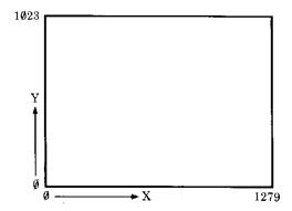
The graphics cursor is an invisible point on the screen, and is where you are about to draw from. Move it about the screen with the **MOVE** command, and drawing is easiest with the **DRAW** command. Thus
