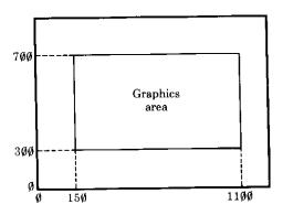
The left hand edge of the graphics area has an X value of (about) 15 $\emptyset$ . The bottom of the area has a Y value of 3 $\emptyset$  $\emptyset$ . The right hand side has X=11 $\emptyset$  $\emptyset$  and the top has Y=7 $\emptyset$  $\emptyset$ . The full statement to set this area is
