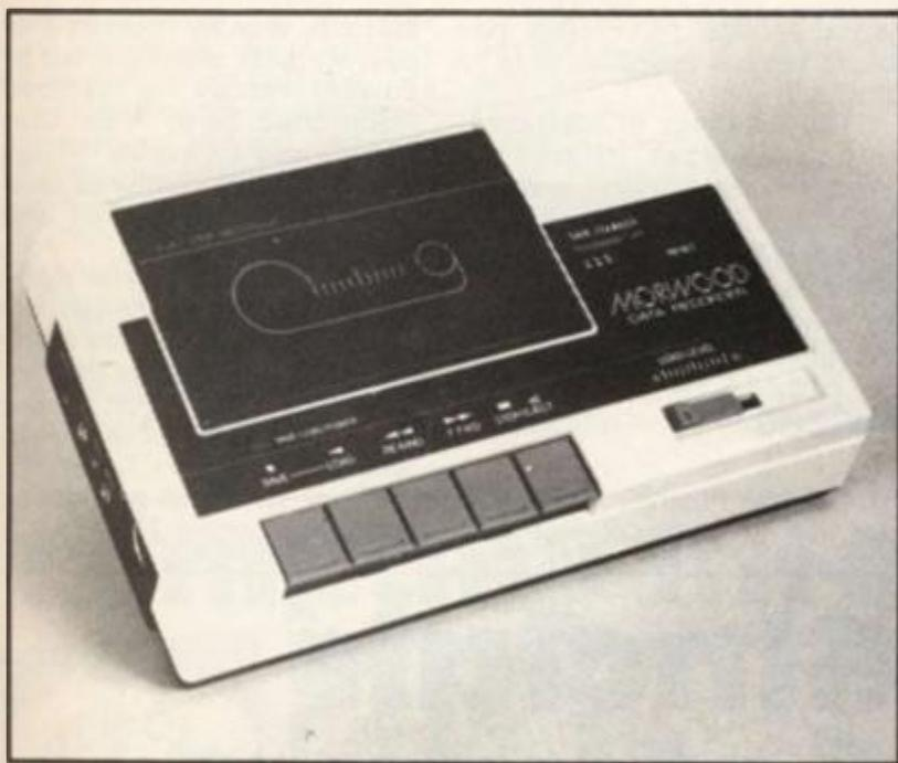
available for an extra £3.00 which will match the load/save signals to the ZX81 by boosting the signal during saving, and the Editor tells me that he tried it out and it worked perfectly for the brief time he had it. Although the head azimuth still needed to be adjusted occasionally on some tapes the signal tone and strength were perfect.
