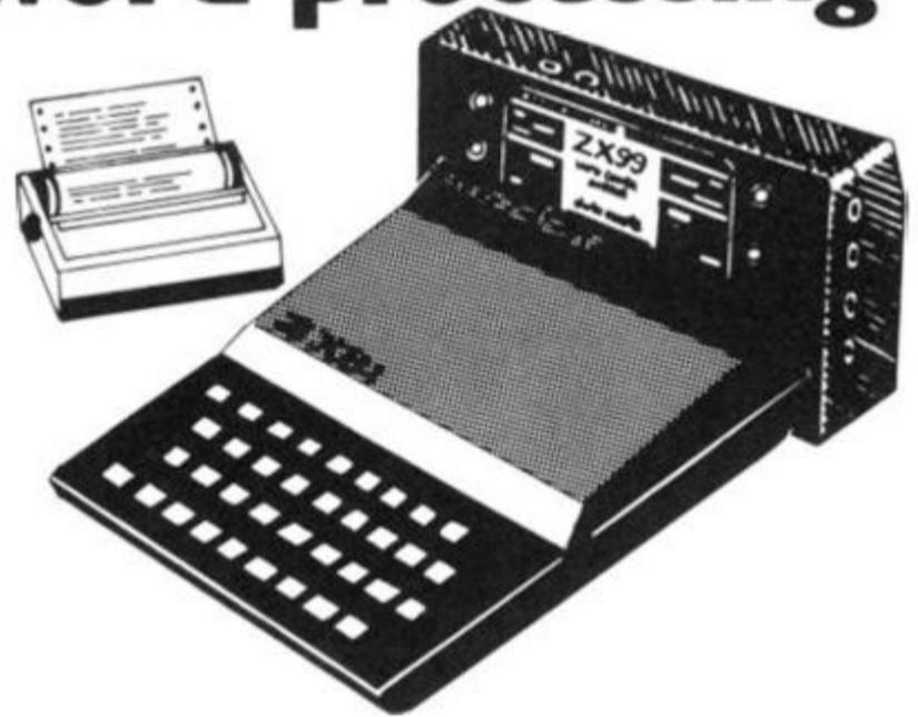
The ZX99 contains its own 2K ROM which acts as an extension to the firmware already resident in your ZX81'S own ROM. The ZX99's ROM contains the tape operating system, whose functions are accessed via Basic USR function calls. Each function has an entry address which must be quoted after the USR keyword. All of the functions can be used in program statements, or in immediate commands (i.e. both statements with line numbers and commands without them).
