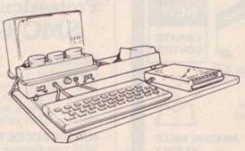
The MICROCARE MICROSTATION is a compact workstation designed to accommodate a ZX81 or Spectrum, Cassette Recorder, Printer, Microdrive with room behind for the BACKPACK of your choice. It is ideal for use in restricted spaces and allows the computer and its peripherals to be moved around with a minimum of effort. Ref. MS £6.00 + £1.50
