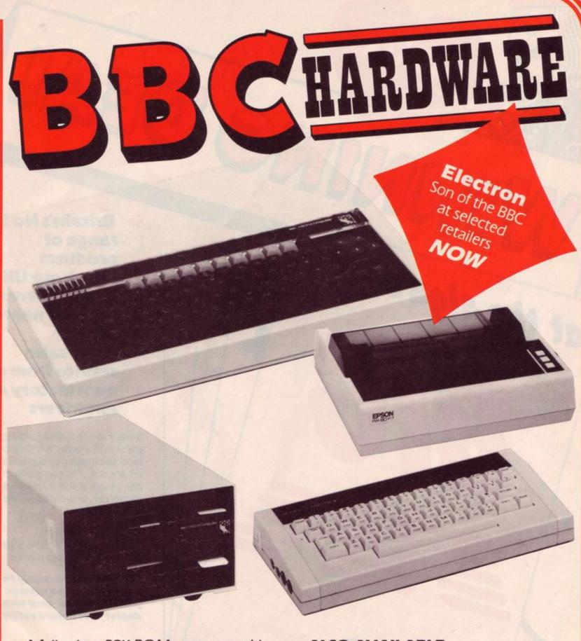
A full colour 32K ROM computer with text and graphics modes up to 640 x 256 graphics and 80 column text screen, extended Microsoft basic, built in assembler 1 MHZ and tube interface, sideways ROM, RS 423, A/D converter.
