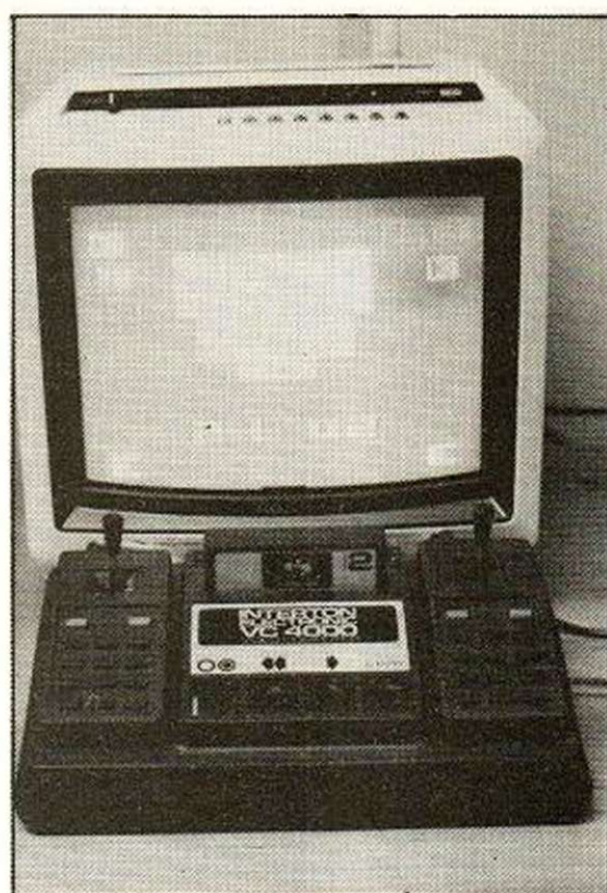
Above: the Interton VC-4000 is based on the same chip as the Acetronic MPU 1000, Radofin 1292/1293, Prinztronic VC-6000, Teleng, Rowtron and Database systems.
