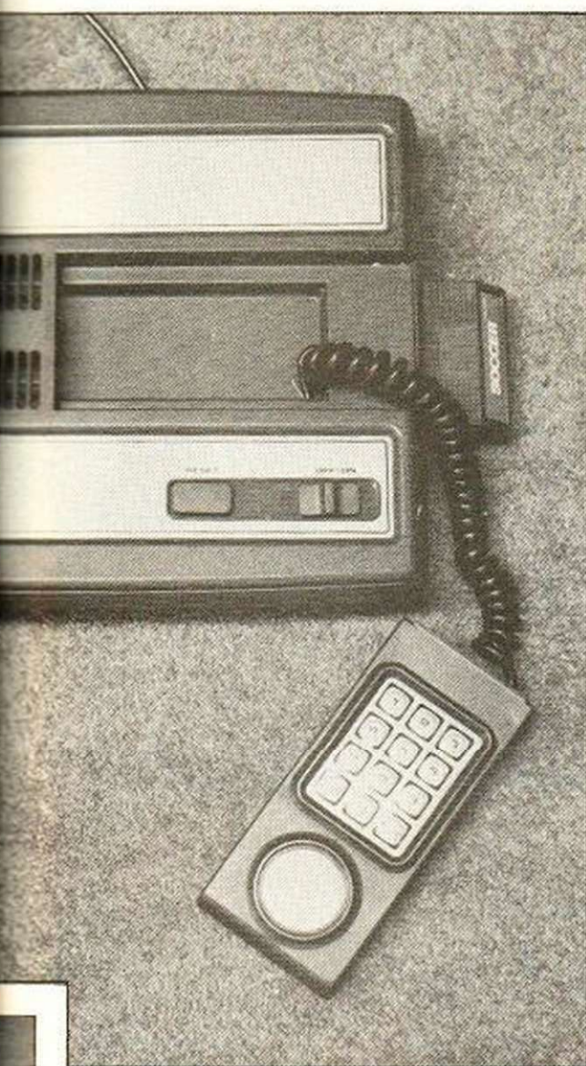
Above: the Interton VC-4000 is based on the same chip as the Acetronic MPU 1000, Radofin 1292/1293, Prinztronic VC-6000, Teleng, Rowtron and Database systems.
