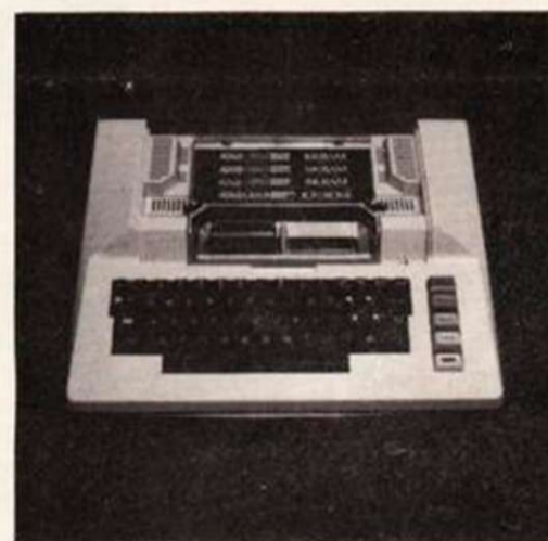
Atari 800 Console (with cover removed)
