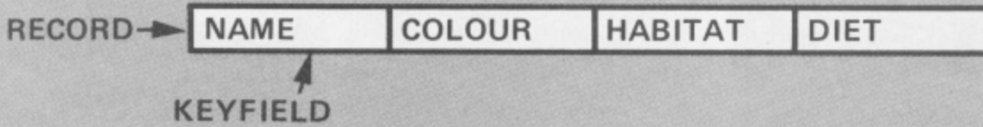
Figure 7.1. Field headings created for a file called "BIRDS". Remember to store the headings along with the information stored under them.
