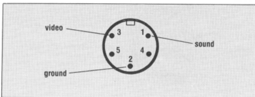
Audio output located on pin 1 of the socket on the Dragon
