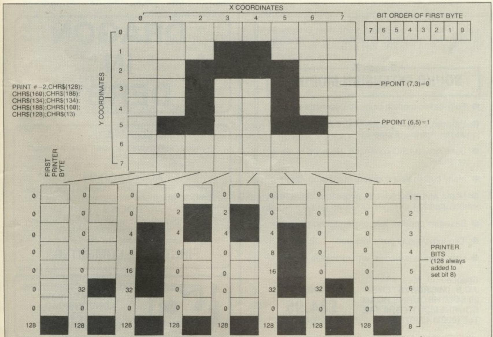
Conversion of a high resolution screen to a GP1000A graphics format
