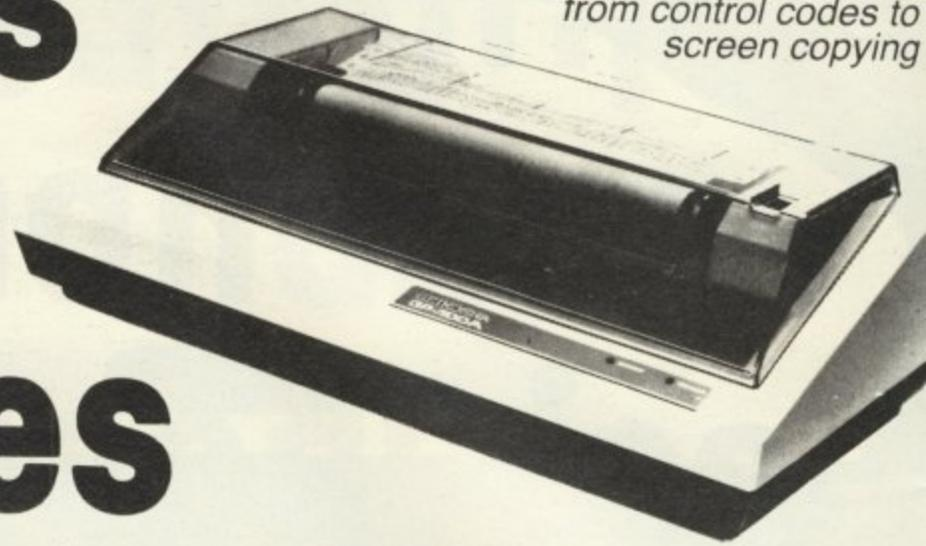
THE SEIKOSHA GP-100A is a versatile and popular low-cost dot-matrix printer with the Dragon-type Centronics parallel interface. It can produce both single and double width character and also has a dot-addressable graphic printing mode.
