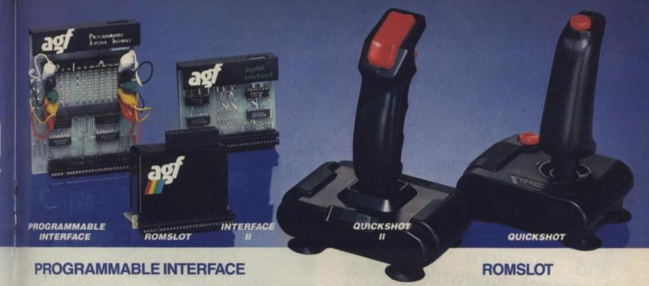
As the first fully hardware programmed joystick interface, this product has become well established over the past year and will accept ALL standard joysticks or trackballs, including Quickshot II with 'rapid fire', for use with ALL Spectrum or ZX81 software — not just those with a joystick option.
