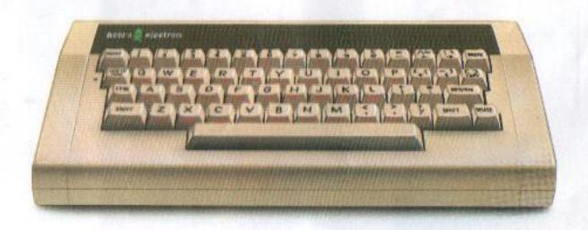
At the heart of the machine lies 64K of memory. Of this, 32K is in the form of ROM (Read Only Memory) containing the Machine Operating System and BASIC interpreter. The other 32K is RAM (Random Access Memory), over 20K of which can be available to you for writing your programs.
