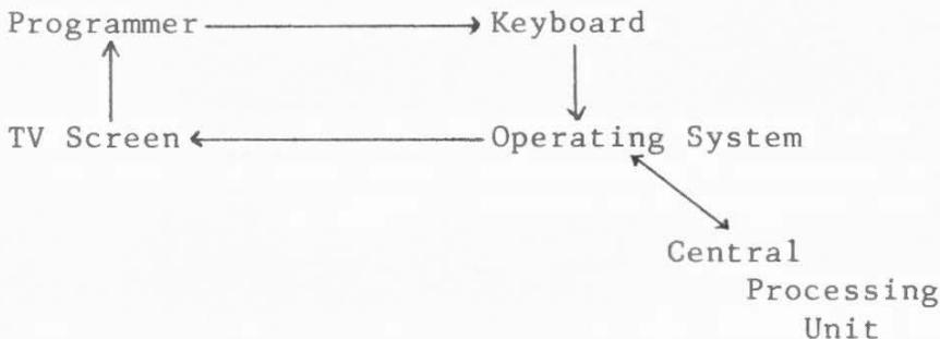
What this diagram aims to show is that there is a barrier between the programmer and the brain of the Spectrum, the Central Processing Unit. It is not possible under normal processing for the programmer to tell the Central Processing Unit - usually referred to as the CPU - what to do.
